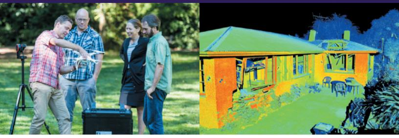
Above left: The UW faculty team tests an Unmanned Ariel System, or drone, that will be used for aerial reconnaissance. Above right: The new center will use state-of-the-art laser equipment to provide detailed scans such as this one, which shows a home damaged by rockfall during the 2011 Christchurch earthquake. The ultra-high resolution helps investigators better understand factors that enhance the resiliency of homes.
